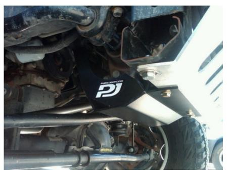
Our skid for the electronic sway-bar found on the Rubicon JK models can be installed with (as shown) or without aftermarket front skid plates. Drilling is required in the stock underrider support to properly mount. On some early model JKs, 1 of the necessary holes will be present. On most applications, all 3 holes will need to be drilled.
